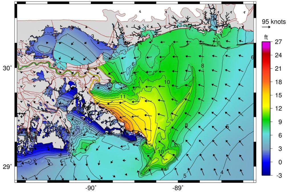
Figure 176: ADCIRC elevation contours (in feet) and wind vectors (in knots) for Hurricane Katrina at 10:00 UTC on August 29, 2005, for Southeastern Louisiana.
